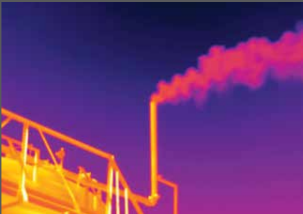
Teledyne's infrared imaging reveals an open vent line in the oil and gas industry.
